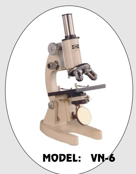
Monocular stable inclinable boothyd horse shoe base, separate coarse & fine motion knobs, fixed eye-piece tube, rack and pinion modienall height 310mm, square stage 110x110mm, triple revolving nosepiece, illumination controlled by iris-diaphragm and condeitser, following optics. but condenser movable by rack and pinion. With this movement of condenser, intensity of light can be and decreased according to the high power and low power objectives for better contrast
